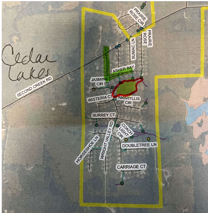
Figure 1: Table Maps depict water flow (green) and reoccurring incidents of flooding (red).
